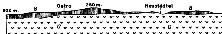
FIG. 57.—Demonstrated profile of the Lausitz granite batholith (G), Germany, which is intrusive into metamorphosed graywackes (S). (Same ref. as for Fig. 56, Sekt. Kloster St. Marienstern.) Horizontal scale, 1:86,000; vertical scale 1:172,000.
